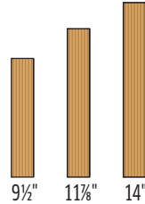
1½" J55-1.6E LVL Floor Joist
